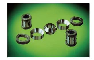
Where stiction may be anticipated or experienced in control valves, Flexitallic offers Enviroflex 503, a specialist product developed with PTFE pockets on the inside diameter of the central olive to further reduce the effects of friction on valve operation.
